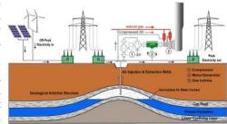
air is expanded to meet peak power needs and air can be stored for long periods of time. Power can also be supplied within minutes.
